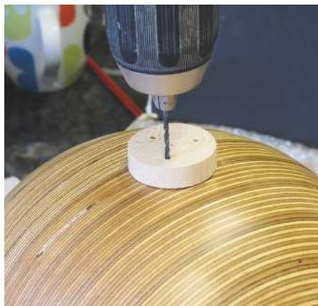
▲ Pic.33 Les made a little jig to allow him to drill the holes in the top for the brass plate. For strength he chose 25mm-long screws
